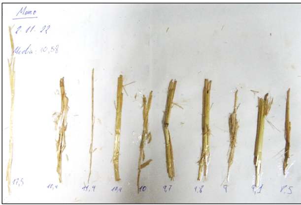
Figure 2. The longest ten fibres of one sample after sieving, straightening and measuring.
